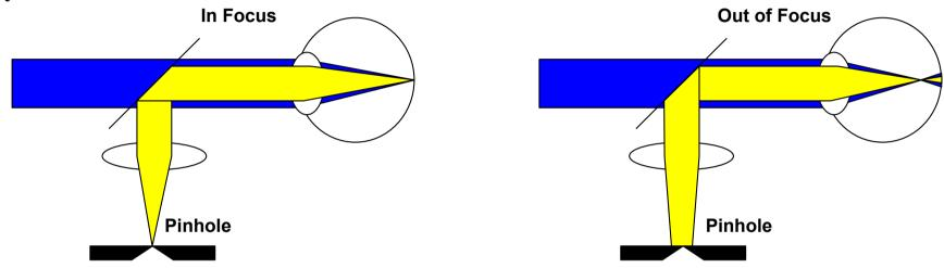
Out-of focus images are not only blurry, they also contain substantially less photons. More than that, the ratio of the good signal and unwanted signals decreases. Therefore the drop in the lifetime accuracy is larger than the drop in SQRT (N).
