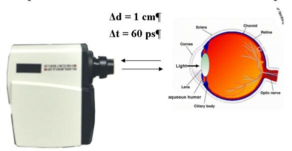
More than 1cm variation during the data acquisition cannot be tolerated. The effect would be a broadening of the IRF (the temporal response function of the system). Data analysis can deliver correct results only if the IRF is correct.
