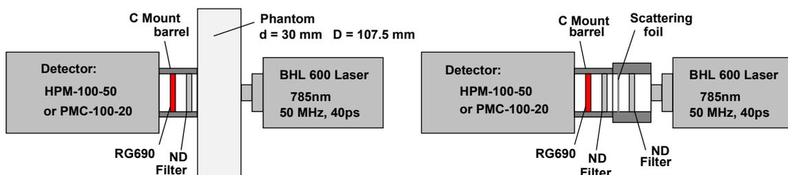
Fig. 1: Test setup. Left: Measurement of time-of-flight distribution in a phantom. Right: Measurement of instrument response function.
