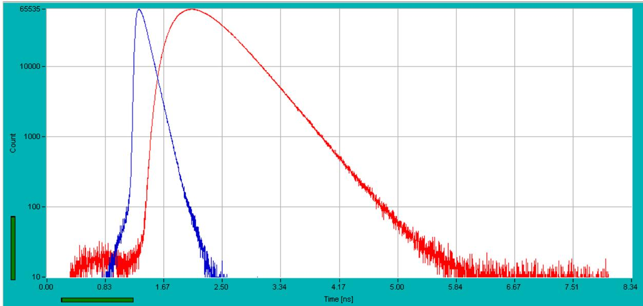
Fig. 2: DTOF (red) measured at the 30 mm phantom and IRF (blue). HPM-100-50 hybrid detector
