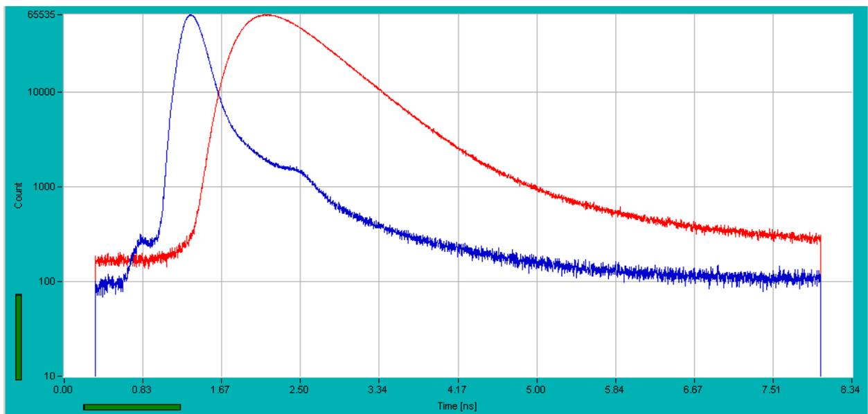
Fig. 3: DTOF (red) measured at the 30 mm phantom and IRF (blue). PMC-100-20 NIR PMT module
